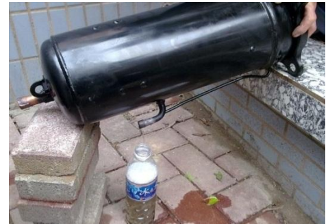
Figure 6-2.5: Draining oil from a compressor
